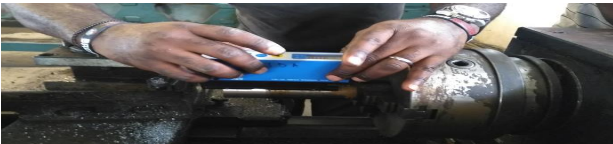
Plate II: The process of measuring surface roughness of turned work piece in an experiment
