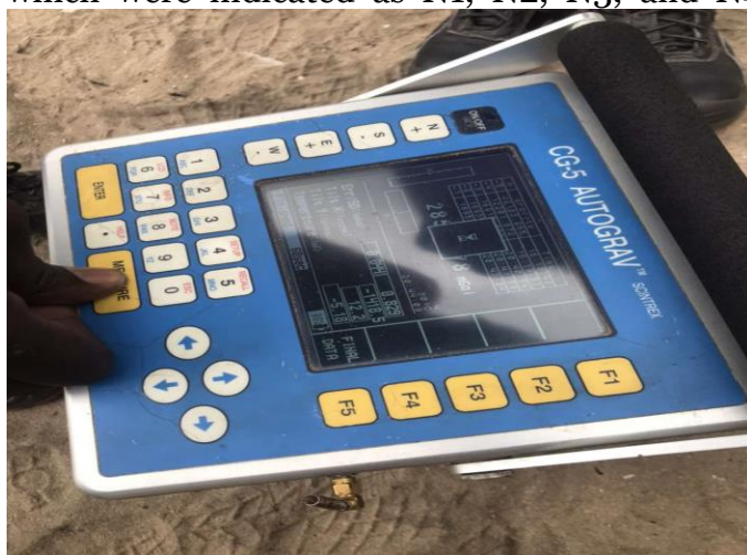
Figure 3.2: CG-5 Autograv meter and other field accessories
