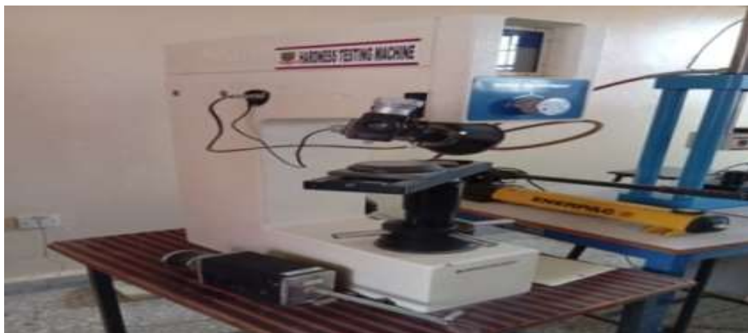
Plate 7 : Brinell Hardness Testing Machine Mechanical Engineering Workshop, NDA, Kaduna.)
