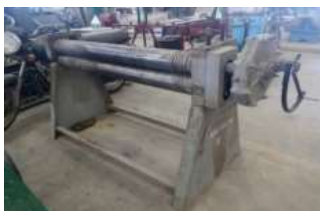
Plate 3: Passing banana pseudostem through mechanical rollers to extract sap
