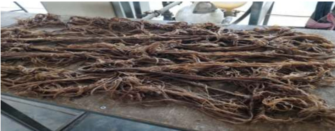
Plate 4: Banana Fibres Dried under Room Temperature for Seven Days
