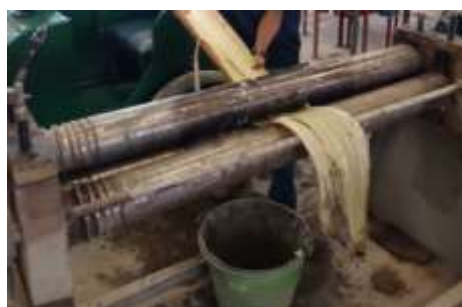
Plate 3: Passing banana pseudostem through mechanical rollers to extract sap
